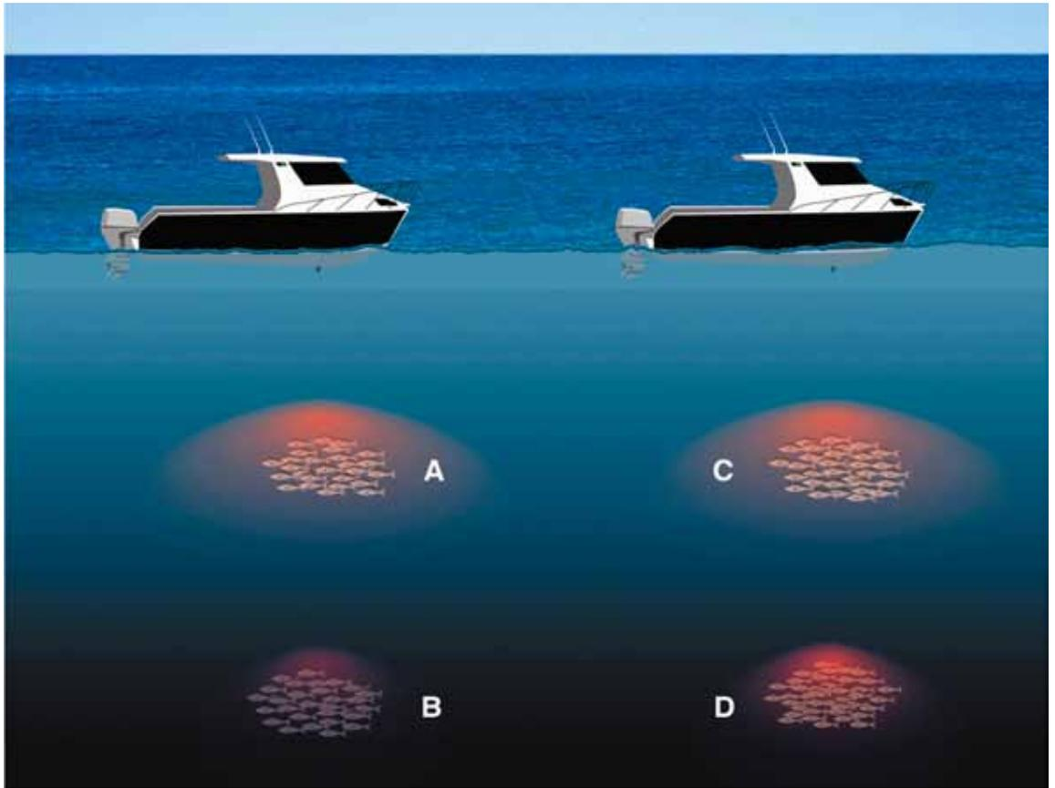
In Figure 43, the TVG is “Off” for the boat on the left hand side and two schools of fish of similar size are located at different depths at A and B. The school of fish at A will produce a stronger echo signal on the display screen than the same size fish school at B. For the boat on the right hand side with TVG “On”, the schools of fish at C and D are recorded proportionally to their size and depth.
